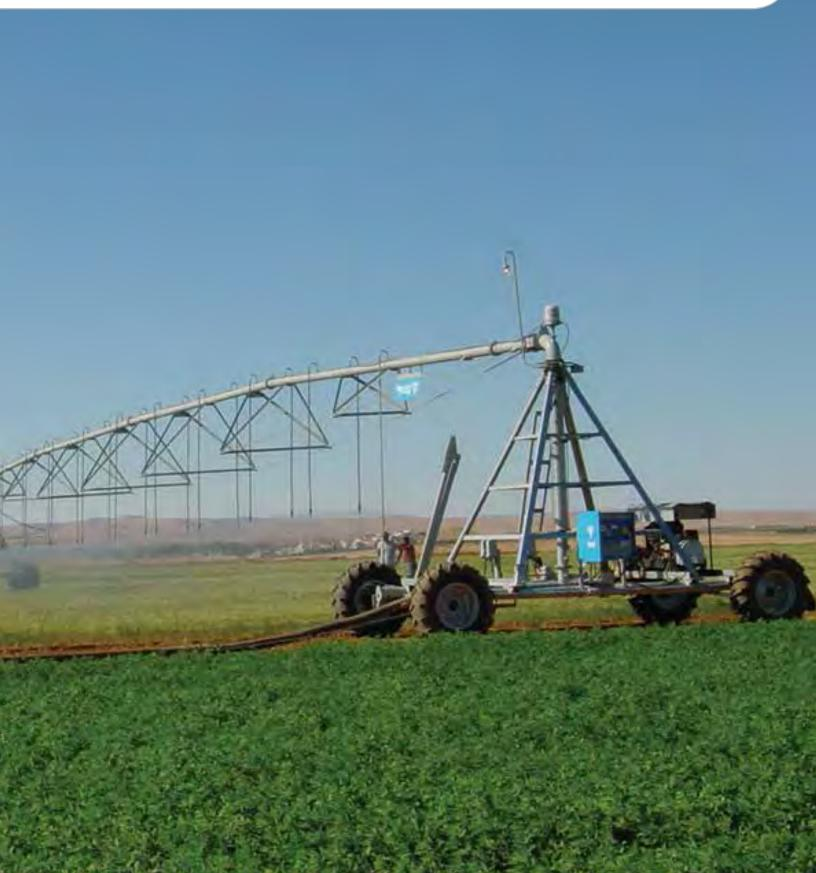
The Valley $_{\odot}$  Universal Linear is engineered for unique field shapes and sizes that require a combination of linear and pivot modes to maximize crop production. The Valley Universal Linear is the only swing-around linear with the ability to automatically switch between linear mode and pivot mode, allowing you to increase your irrigated hectares.
